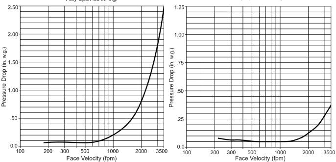
Typical performance for Model GI850 backdraft damper size tested 42"W x 42"H, furnished with counterweight to assist opening.
